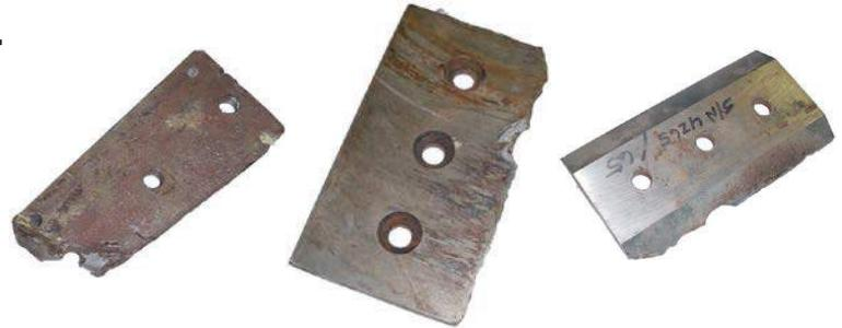
Shown here: Damaged chipper knives
